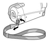
Pass the attaching end of the wrist strap through the back bracket on the camcorder, thread the wrist strap through the loop and fasten.
